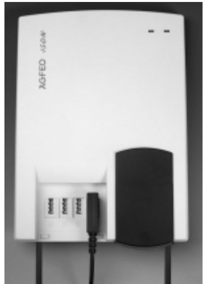
Fig. 4: Telecommunications system with plugged power supply, ISDN access and TAE plug
